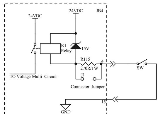
**Note:** 1 Factory default disconnect the internal jumper J1. When the Safe Lamp needs to be connected, it needs to connect the internal jumper J1.
